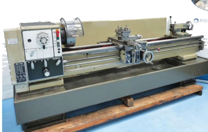
Harrison M400 80in Gap Bed Centre Lathe 80in (2,000mm) between centres, 16 1/2in (420mm) swing 24 1/2in (610mm) in gap, 65mm bore, taper turning. £10,750
